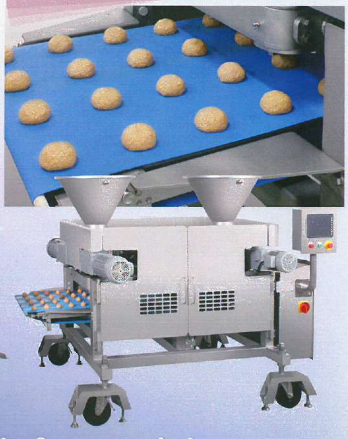
Four Rows Encrusting Model Producing 48,000 pcs / hour
