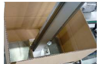
Mechanical plunger for perfect bonding
