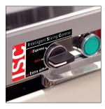
Intelligent Slicing Control (JAC patent) Continuous automatic control system that Slices loaves according to their consistency. This allows open textured, crusty and dense breads to be sliced with equal efficiency.
