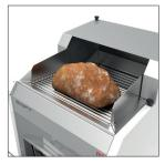
Multiformat loaf front loading area. The loading area consists of rollers on ball bearings to automatically direct loaves to the loaf changeover area. Given that it is located facing the operator, this simplifies the handling of loaves considerably. It is not necessary to make adjustments for different loaf formats, as the slicer adapts, saving you time and improving ergonomics.
