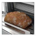
Sliced loaf delivery area. The delivery area is located at the correct height to facilitate the handling of loaves sliced. As it is provided with holes, any crumbs fall into the recovery tray.
